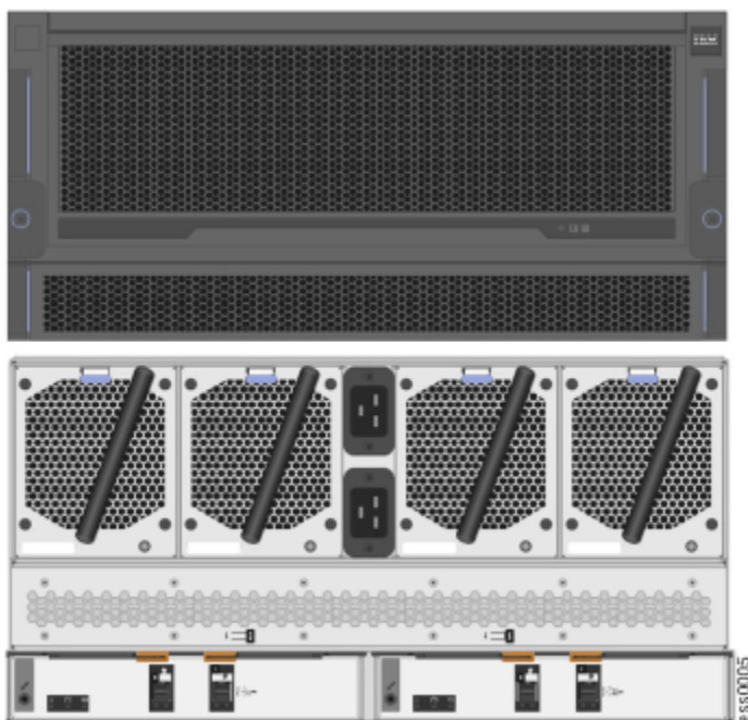
Figure 5. Front and rear view of Model 092 expansion enclosure
